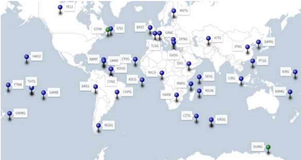
Figure 1. Network of Regina stations. Green: standard station, not E6 GALILEO compatible. Blue: newest generation station, E6 GALILEO compatible.
